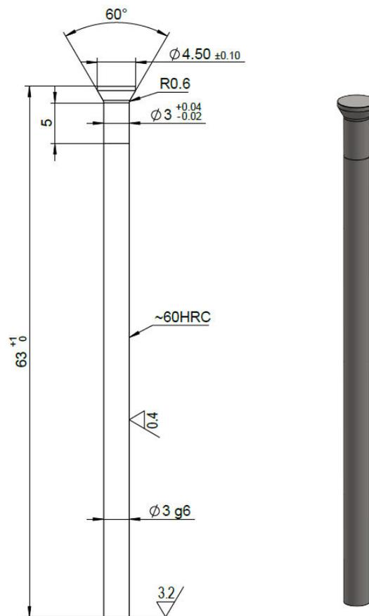
Fig.11.2.: Dowel pin DP-3g6-63 dimensions
