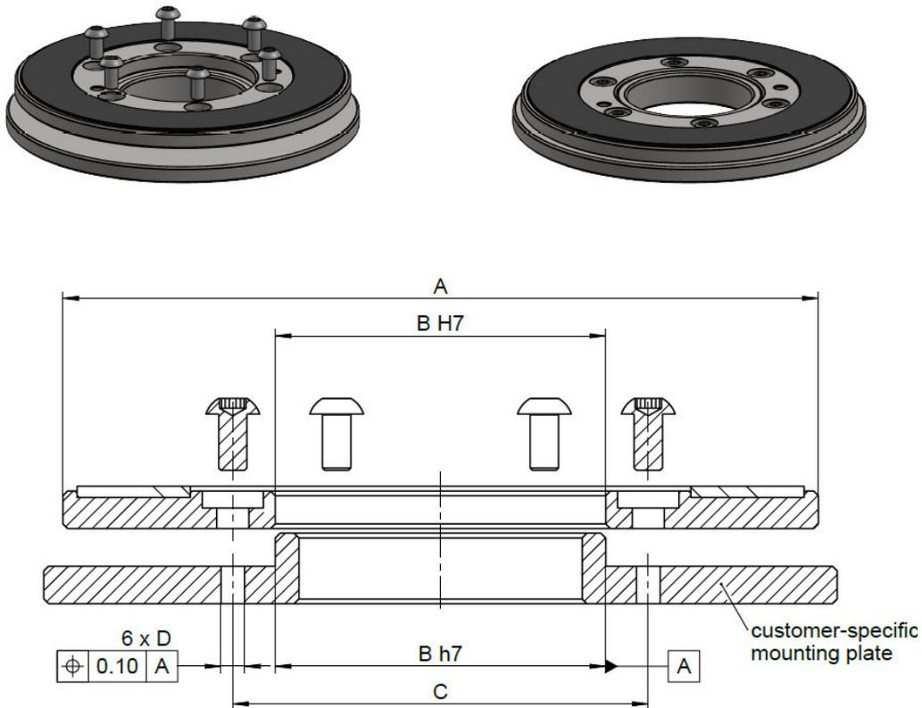
Fig.4.2.: Rotor (GAR) mounting using ID sliding fit
