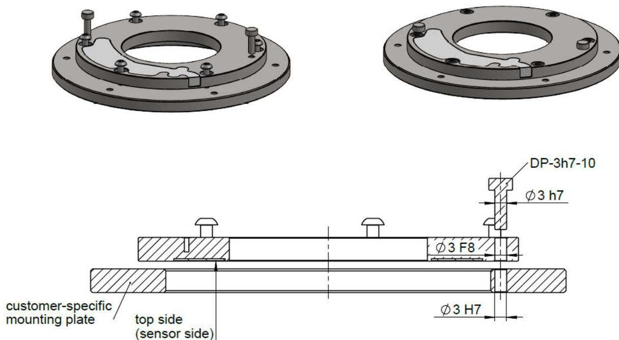
Fig.4.5.: AMH Dowel-Pin mounting
