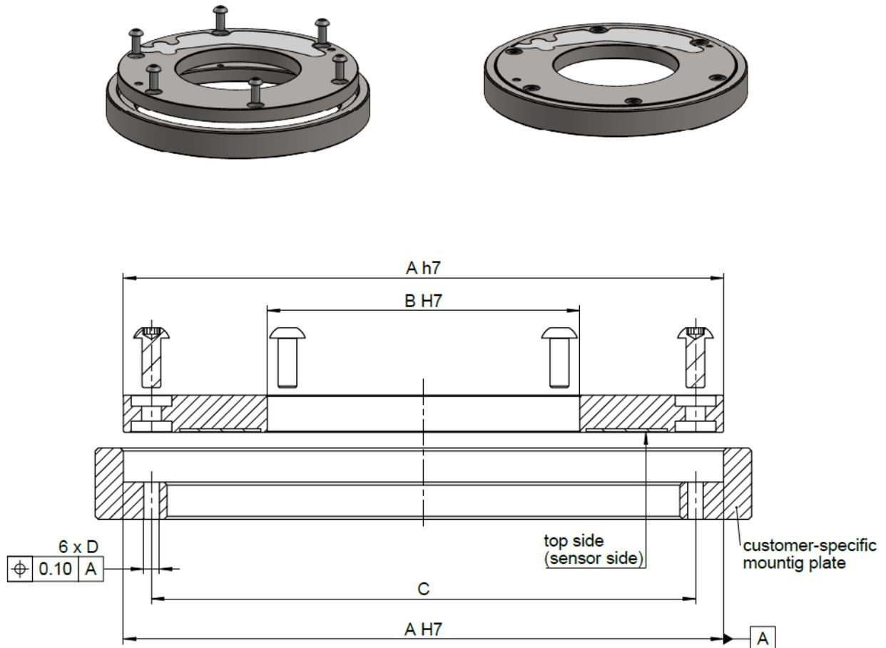
Fig.4.3.: Stator (GAS) mounting using OD sliding fit
