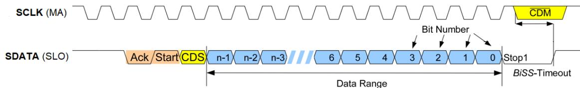
**“Ack” bit is always 1 Clock length for all FLUX encoders.**
