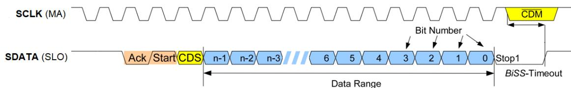
**“Ack” bit is always 1 Clock length for all FLUX encoders.**
