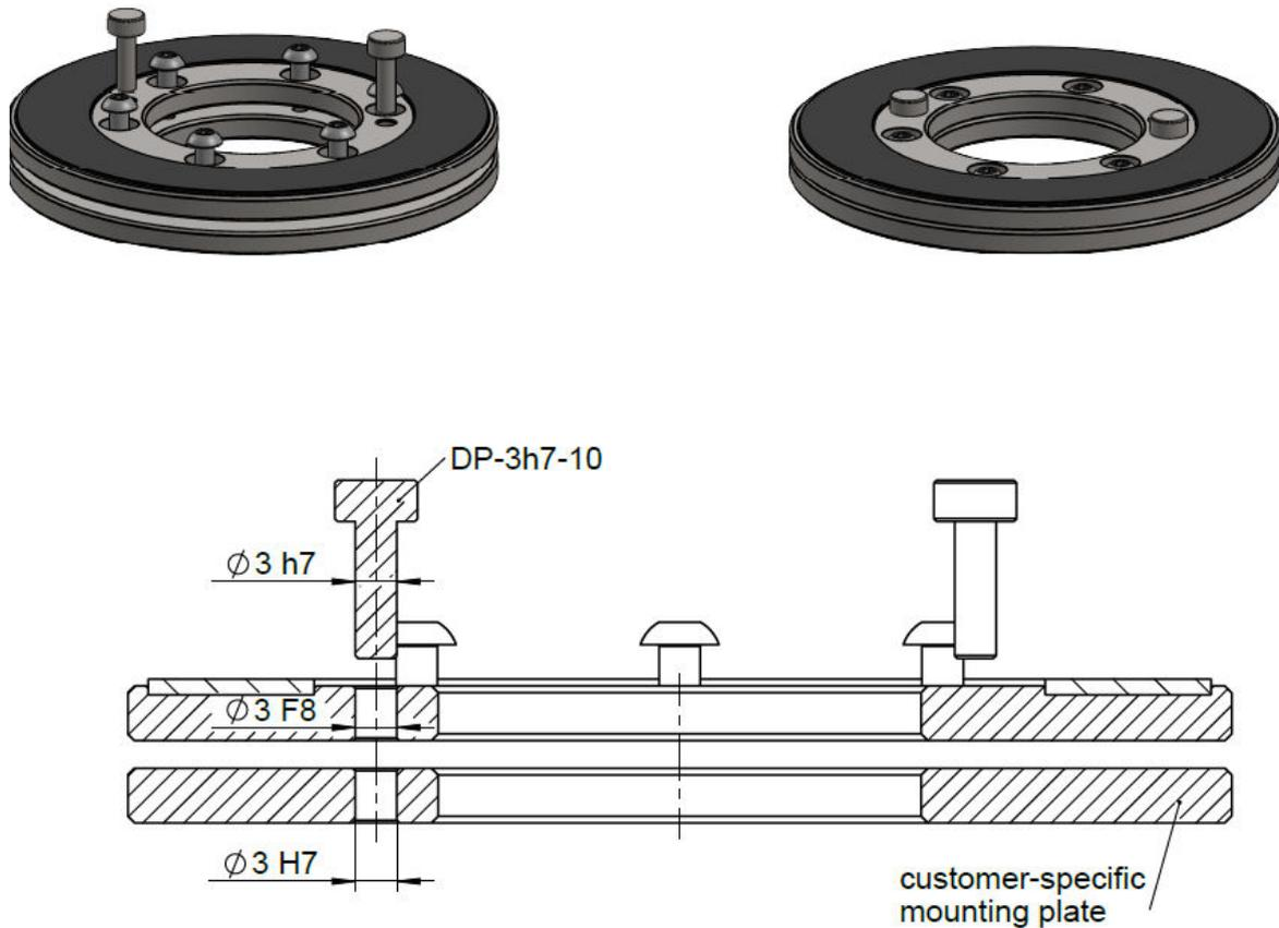
Fig.4.6.: AMR Dowel-Pin mounting
