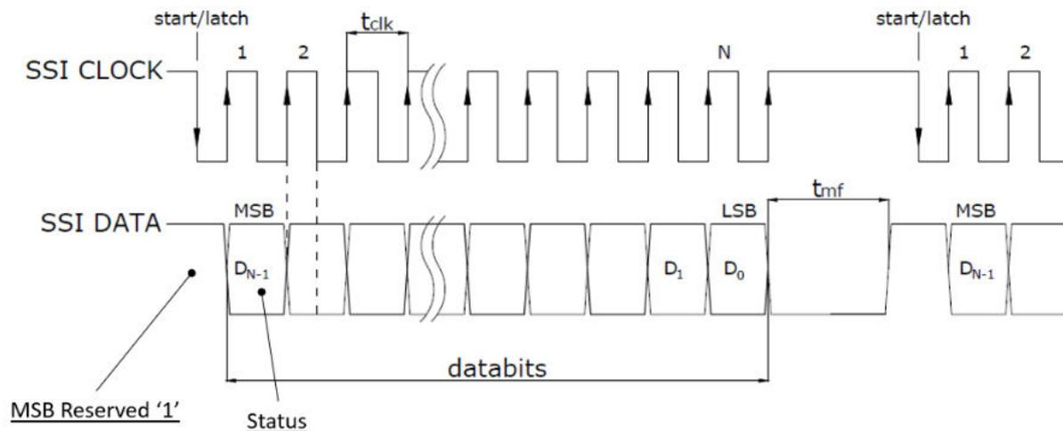
Fig.5.4.: Time Diagram for the SSI02 interface
