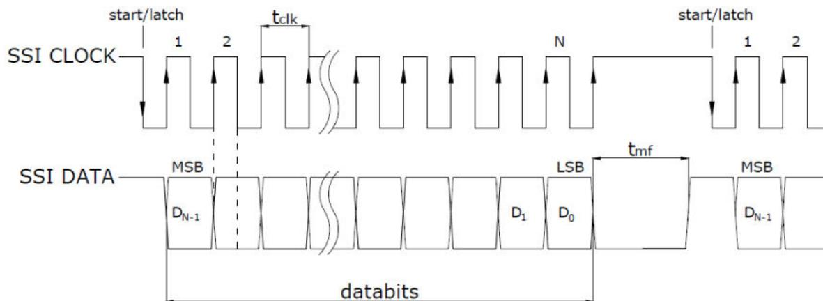
Fig.5.2.: SSI01 time diagram
