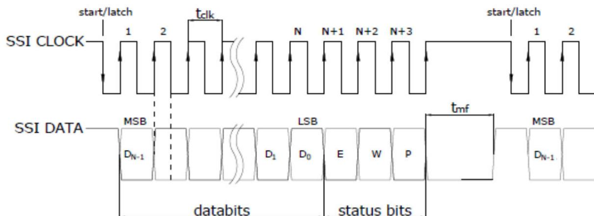
Fig.5.1.: SSI00 time diagram
